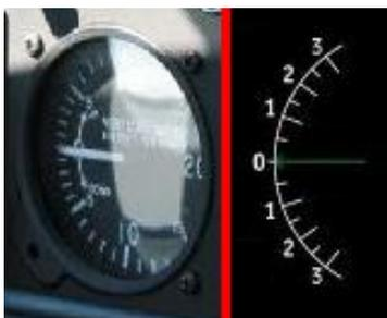
*Vertical Speed Indicator (VSI) or Vertical Velocity Indicator (VVI) or Rate of Climb Indicator*
