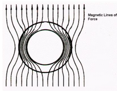
When a signal is applied, the magnetic lines of force from the earth are forced out of the permiable core of the flux valve transformer.
