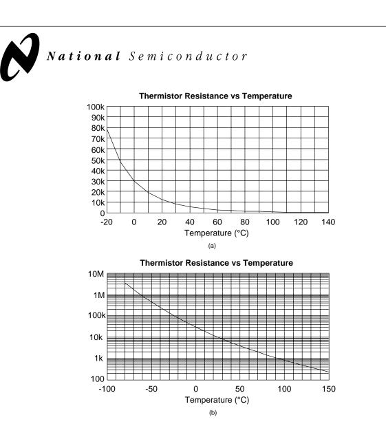
Figure 2.2. Thermistor Resistance vs. Temperature. (a) linear scale. (b) logarithmic scale.
