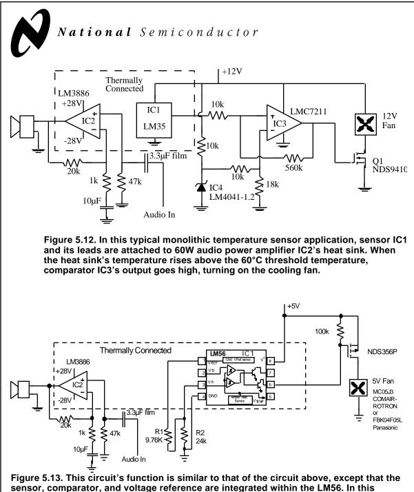
circuit, the fan turns on at 80°C and off at 75°C.
