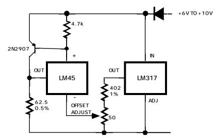
Figure 5.15. 4-20mA Current Transmitter Temperature Sensor
