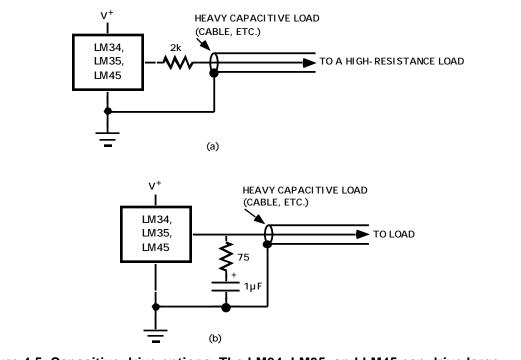
Figure 4.5. Capacitive drive options. The LM34, LM35, and LM45 can drive large external capacitance if isolated from the load capacitance with a resistor as in (a), or compensated with an R-C network as in (b).
