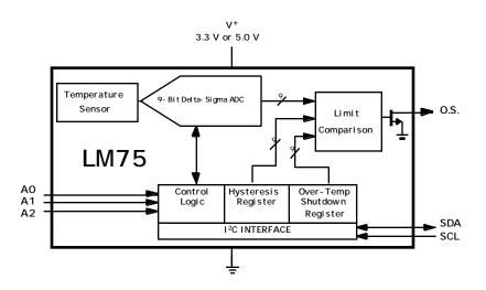
Figure 3.7. LM75 Block Diagram.
