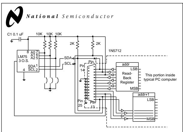
Figure 5.6. PC-Based Temperature Acquisition via the Parallel Printer Port.
