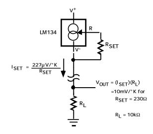
Figure 3.5. LM134 Typical Connection.  $R_{\mbox{\tiny SET}}$  controls the ratio of output current to temperature.
