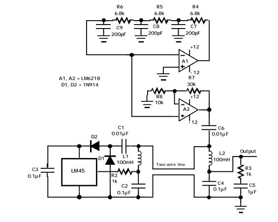
Figure 5.14. This two-wire remote temperature sensor transmits the dc output of the sensor without reducing its accuracy.
