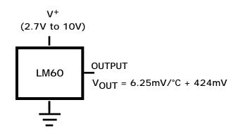
Figure 3.4. LM60 Typical Connection
