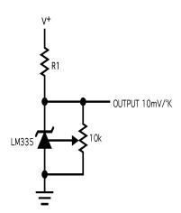
Figure 3.1. Typical Connection for LM135, LM235, and LM335. Adjust the potentiometer for the correct output voltage at a known temperature (for example 2.982V @ 25°C), to obtain better than  $\pm 1^{\circ}$ C accuracy over the -55°C to +150°C temperature range.
