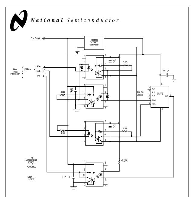
Figure 5.7. Isolated PC-Based Thermometer.
