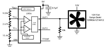
Figure 5.3. You can control some fans without adding a power device to the system. This circuit controls a fan's speed by taking a "third lead" low when temperature is high. This increases the fan's speed to provide additional cooling.
